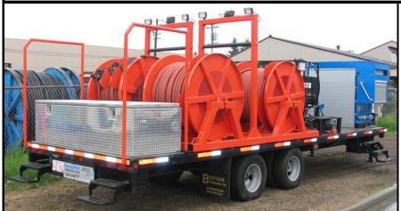
This self-contained powered cable reeler is designed to carry 4 reels of electrical distribution type cable for emergency dispatch. The reeling units are securely mounted on a heavy duty steel chassis designed to be towed behind a 1 ton (or larger) vehicle. The diesel engine provides sufficient power to reel all 4 reels at once, and is controlled by the handheld remote control. Each reeling unit has a built-in disc brake, which is spring loaded to ensure reels don't rotate during transport.
