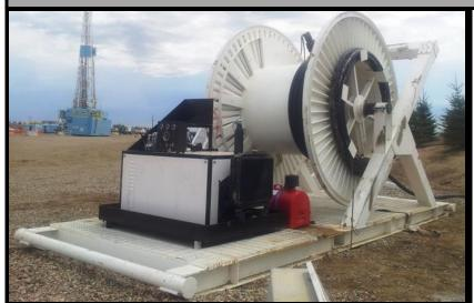
This cable reeler is designed as a portable unit with a fixed, non-removable cable reel and adjustable speed level wind. This unit is powered by a 40 HP diesel engine to operate the gear/sprocket/chain drive. Built on a 20 ft long skid, this reeler is designed to payout and take up 2500 ft of 25kV, 1/0 SHD-GC power cable, for a maximum payload of 17,000 lbs. The cable reel on this unit is designed with brackets on the outer rim to hold termination pigtails up to 20 foot length.
