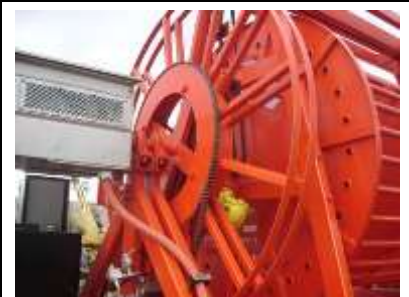
Monospiral reel with slip ring connection
