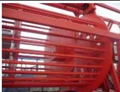
Vented, open style reel to allow for air circulation
