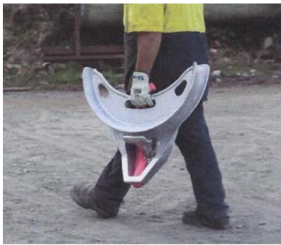
Cable Handling Grab: Light weight,
