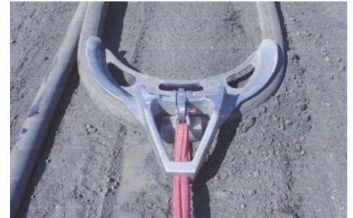
Maintains minimum safe cable radius.
