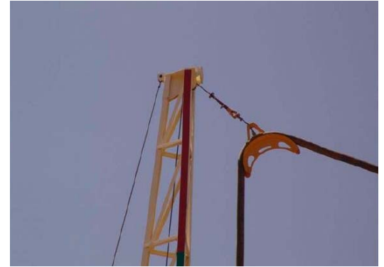
Cable Grab suspended with Safety Sling
