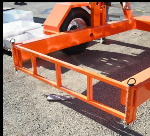
Rear gate to enclose cable reel
