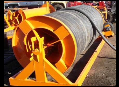
Above: Rail Mounted Cable Reeler, designed for mounting on tracks inside an underground tunnelling operation to feed TBM's
