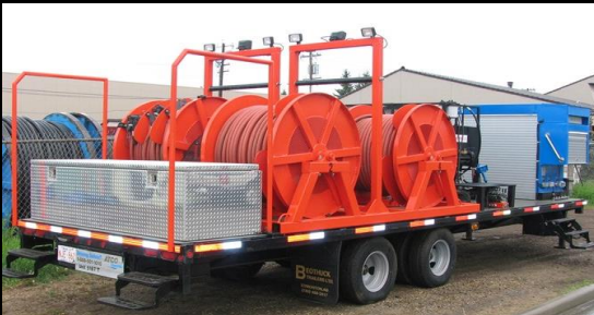
Above: Shore Based Cable Reeler with dielsel hydraulic power pack. Includes wired remote control, disc brakes, and level wind. Designed for 3000 ft of 5kV, 2/0 SHD-GC cable, interchangeable reels, and a max. payload of 20,000lbs.
