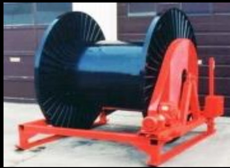
Above: Chain and sprocket driven, fixed reel cable reeler. Light and portable for easy movement in and around your cable repair facility. Powered by single phase, 240V, 5HP motor via reduction gearbox.
