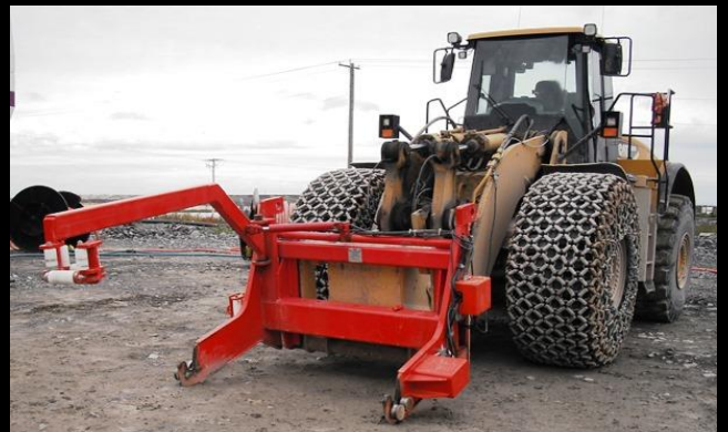
Left: Energized Slip Ring Cable Reeler. Designed to reel 1000ft of 8kV cable in one direction, and 150ft of 8kV cable in the other. Maintains constant cable tension to payout or take up cable without operator input. Self contained hydraulic power unit is powered from onboard cable via a transformer with optional wireless remote control to operator if manual operation is required.
