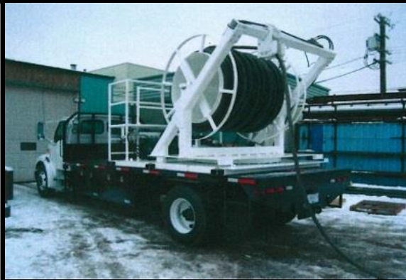
Left: Truck Mounted Cable Reeler with self contained diesel hydraulic power pack. Reel is mounted on a slew bearing, allowing 180° rotation. Includes wireless remote control and level wind.
