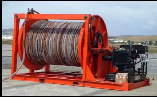
Above: Shore Based Cable Reeler with dielsel hydraulic power pack. Includes wired remote control, disc brakes, and level wind. Designed for 3000 ft of 5kV, 2/0 SHD-GC cable, interchangeable reels, and a max. payload of 20,000lbs.
