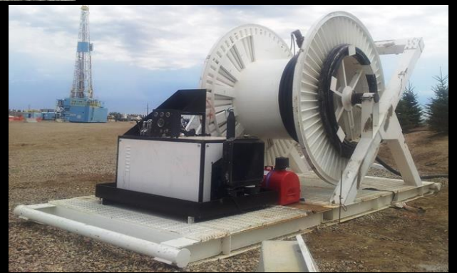
Left: Energized Slip Ring Cable Reeler. Designed to reel 1000ft of 8kV cable in one direction, and 150ft of 8kV cable in the other. Maintains constant cable tension to payout or take up cable without operator input. Self contained hydraulic power unit is powered from onboard cable via a transformer with optional wireless remote control to operator if manual operation is required.
