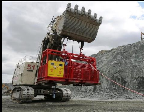
Left: Energized Slip Ring Cable Reeler. Designed to reel 1000ft of 8kV cable in one direction, and 150ft of 8kV cable in the other. Maintains constant cable tension to payout or take up cable without operator input. Self contained hydraulic power unit is powered from onboard cable via a transformer with optional wireless remote control to operator if manual operation is required.
