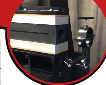
Mine Cable Services recommends the addition of the heavy duty rolling Vulcanizer Cart with the Hydraulic Cable Repair Vulcanizer, providing a complete unit, together providing easy portability within your cable repair shop, allowing movement of the vulcanizing equipment to your cable rather than maneuvering repaired cable to the vulcanizer. See ordering information below.
